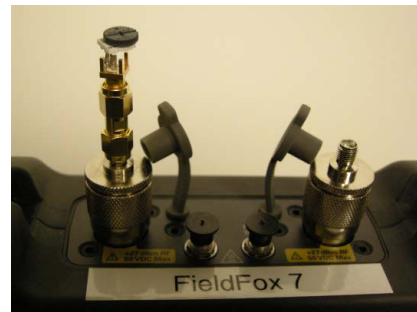
Figure 6. Connection of the 500 \Omega potentiometer load
