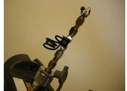
Figure 10. Final assembly of the matching network and the experimental load
